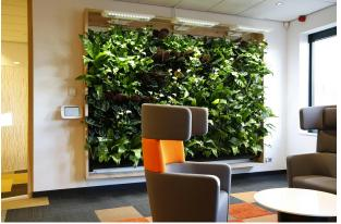
Marrying nature and technology, Lune will present Cloud Garden, which monitors and improves the indoor climate of airports by harnessing the natural air filtration properties of plants. With a 'green wall' at its center, it can transform an airport terminal's atmosphere, both visually and in terms of air quality
