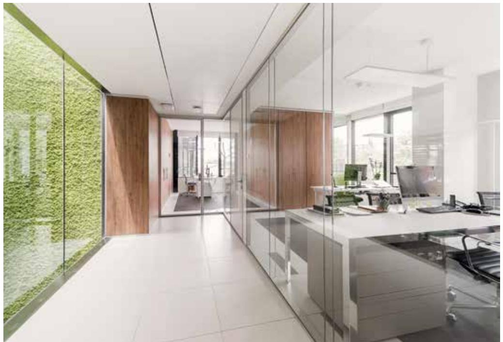
**W80 is a partition wall with a total thickness of 80 mm available in the following versions: glass partition (double or single glazing flush with the exterior) and solid partition (wood, melamine and fabric).**
