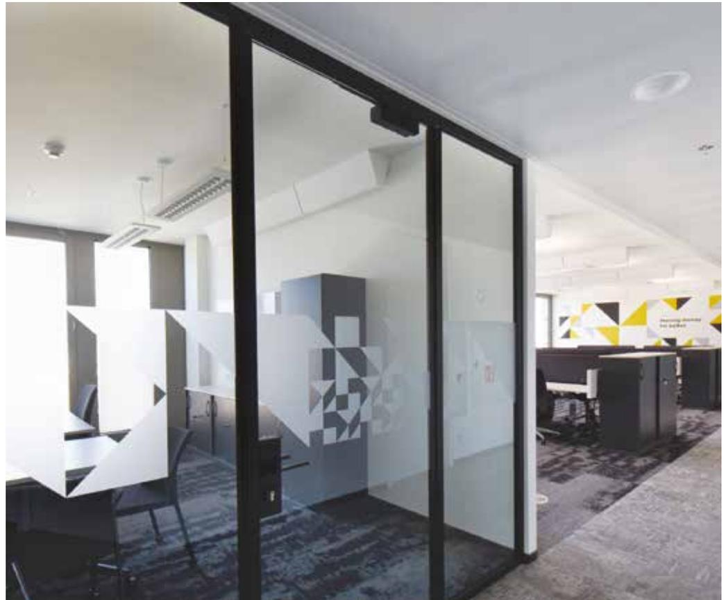
**WE is a single glazed partition wall with a total thickness of 45 mm 1" 3/4. Its simplicity and elegance make it suitable for dividing operational spaces. Its high-tech appeal stems from Cric (jack), the patent pending foot which makes for easier assembly and glazing adjustment**
